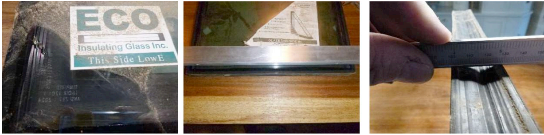
Photos 34, 35, 36: The etched markings, the inward curved spacer compared to the ruler and the inward shaped secondary sealant.
